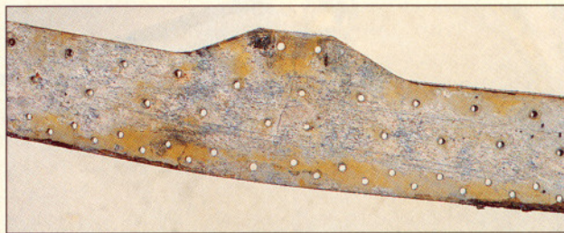
Replacement of defective wing spar caps involves disassembly of the wings, removal of the fuel cells, and new spar caps and straps. Strap below shows the effects of dissimilar-metals corrosion.
